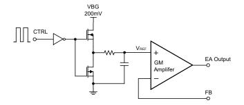
Figure 3. Programmable FB Voltage Using PWM Signal
