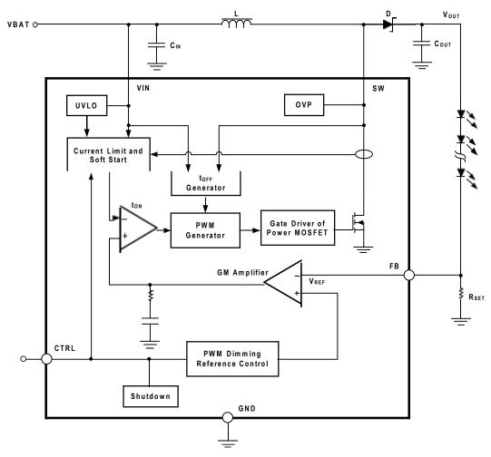
Figure 2. Block Diagram
